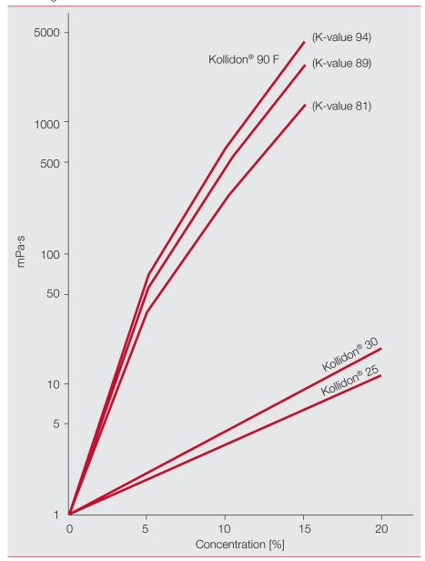
Fig. 1: Viscosity of Kollidon® solutions (Ubbelohde viscometer, 25 °C)
