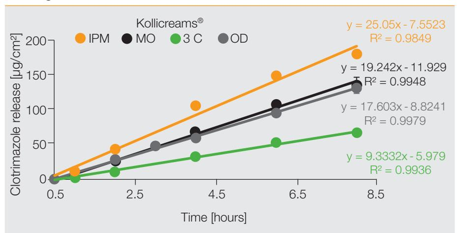
Figure 5: Time profiles of Clotrimazole permeation through a model membrane for different emollients: IPM = Kollicream® IPM, MO = Mineral Oil, 3 C = Kollicream® 3 C, OD = Kollicream® OD.
