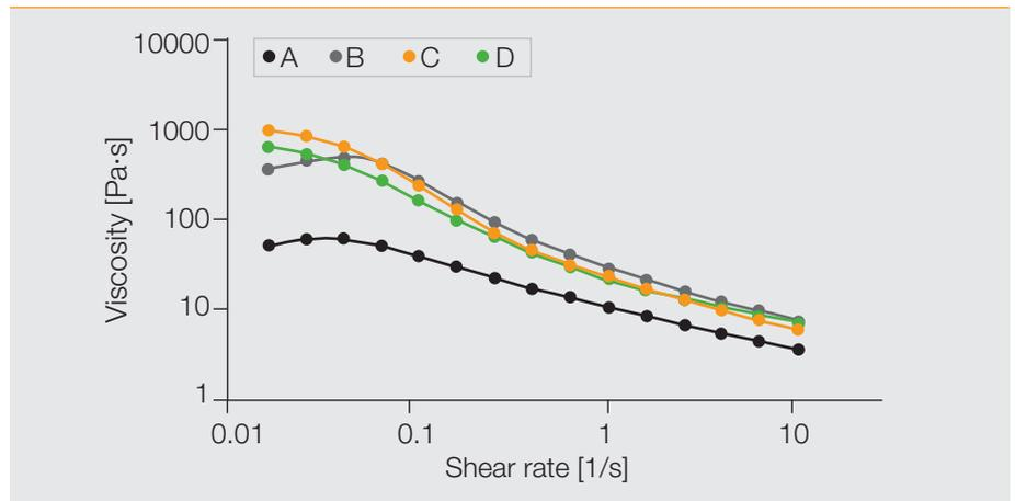
Figure 6: Viscosity profiles of aerosol foams.
