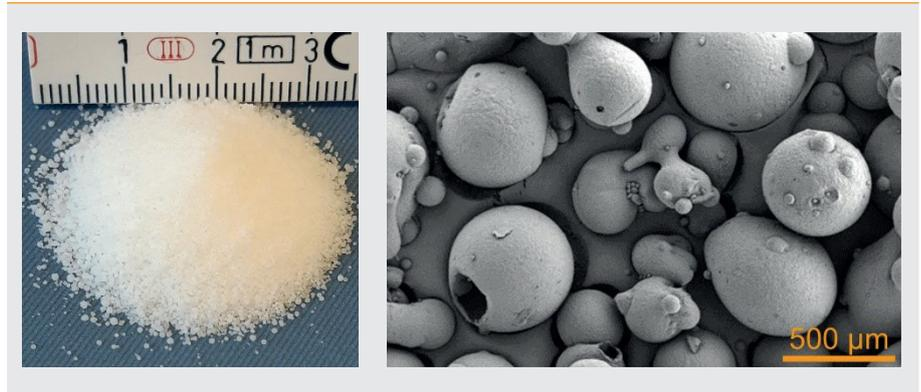
Figure 2: Kolliwax® GMS II is provided as a free-flowing powder (left), consisting of spherical particles that are formed during the spray crystallization process. These structures can be seen in the scanning electron microscope image (right).
