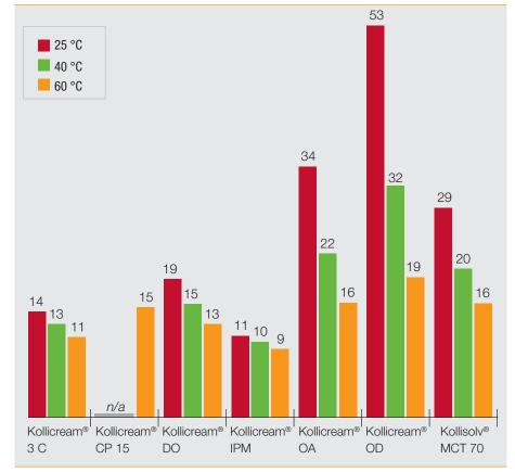
Figure 2: Brookfield Viscosities (values given in cP), measured at three different temperatures. Due to the relatively high melting point, Kollicream<sup>®</sup> CP 15 could not be measured at the first two temperatures.
