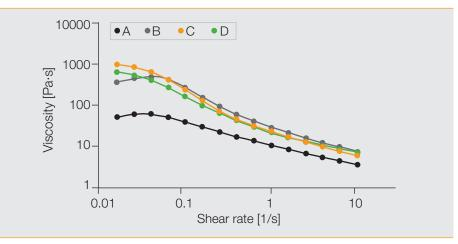
Figure 6: Viscosity profiles of aerosol foams.
