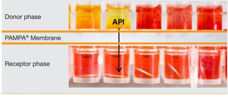
Figure 4: Cutout of the PAMPA setup for the measurement of API penetration through model membranes. The setup allows 96 parallel measurements.
