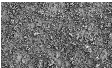
Fig. 2: Scanning Electron Microscopy Pictures ( magnification: 50 ) of Kollidon® CL, Kollidon® CL-F and Kollidon® CL-SF
