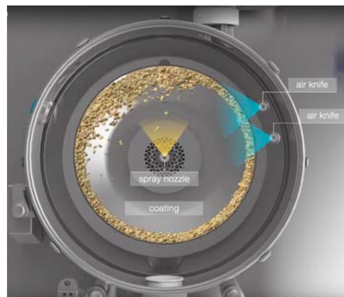
Figure 2. Design of the ConsiGma® coater, used in the present case study.
