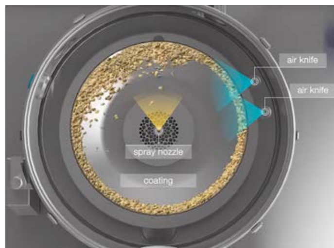
Figure 1. Design of the ConsiGma® coater, used in the present case study.
